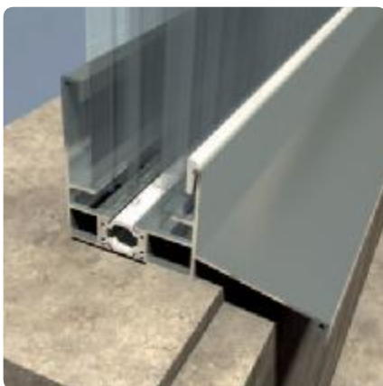
BASE PROFILE WITH TT Detail base profile TT with eave in AL
