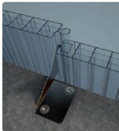
INSERTION OF PLATE Insertion of stainless steel plates for anchorage to existing structures.
